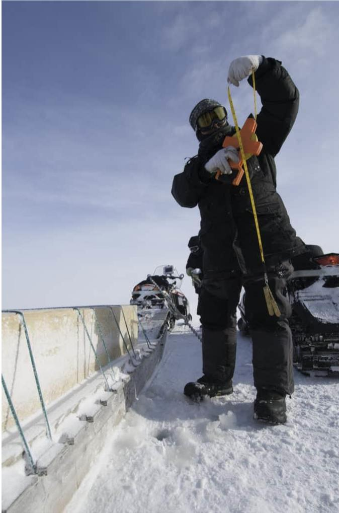
Rex Holwell calibrates the SmartKamutik, to ensure the radar reading and actual ice thickness are approx. the same.
